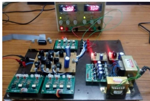
Figure.7 Hardware Setup of 17-Level Proposed Topology
