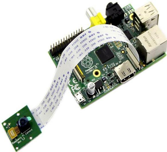
Figure3: Pi Camera Connection on Raspberry Pi
