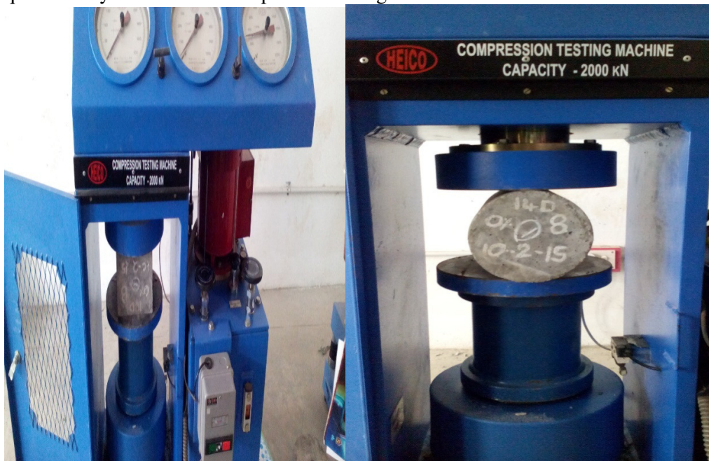
Fig 4.7 Testing of concrete compressive strength
