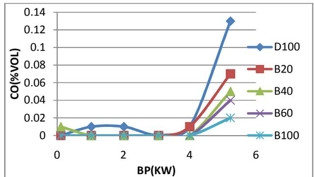
Fig -5(b): Variation of carbon monoxide with brake power with EGR
