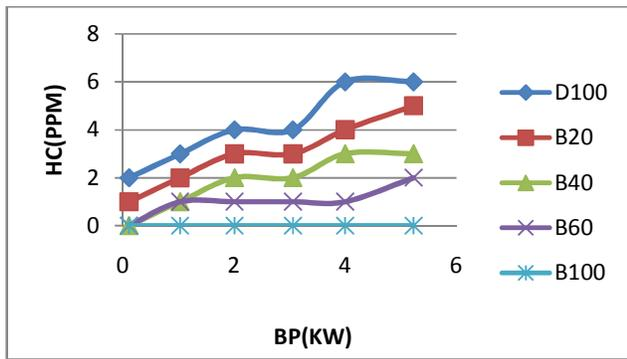
Fig -6(b): Variation of hydrocarbon with brake power and EGR.
