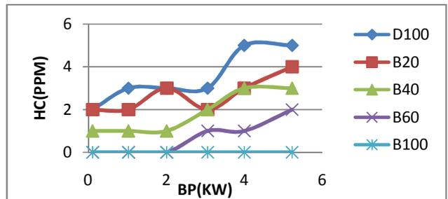
Fig -6(a): Variation of hydrocarbon with brake power and without EGR.
