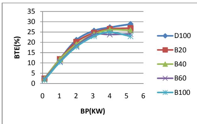
Fig -2(a): Variation of brake thermal efficiency with brake power without EGR
