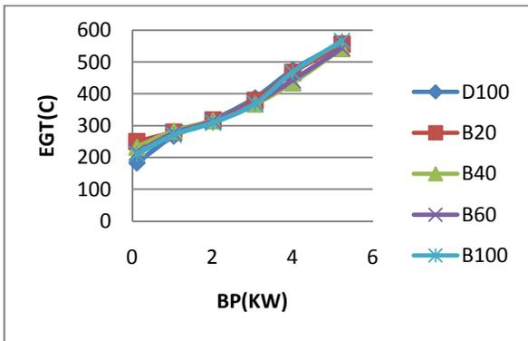
Fig -4(b): Variation of exhaust gas temperature with brake Power with EGR
