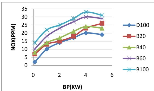
Fig -7(b): Variation of NOx with brake power with EGR
