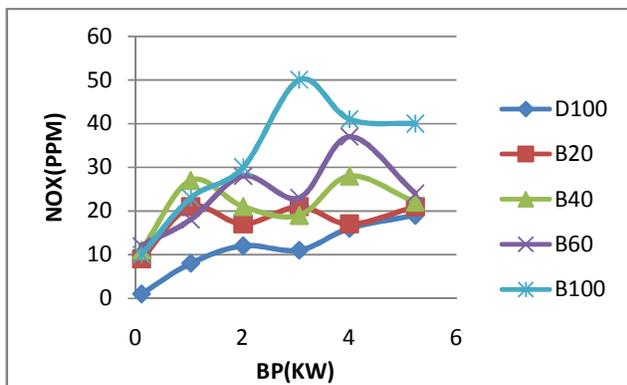
Fig -7(a): Variation of NOx with brake power without EGR
