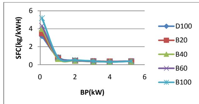
Fig 3(b): Variation of specific fuel consumption with BP with EGR
