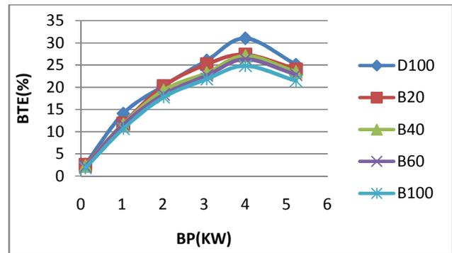
Fig -2(b): Variation of brake thermal efficiency with brake power with EGR(5%)
