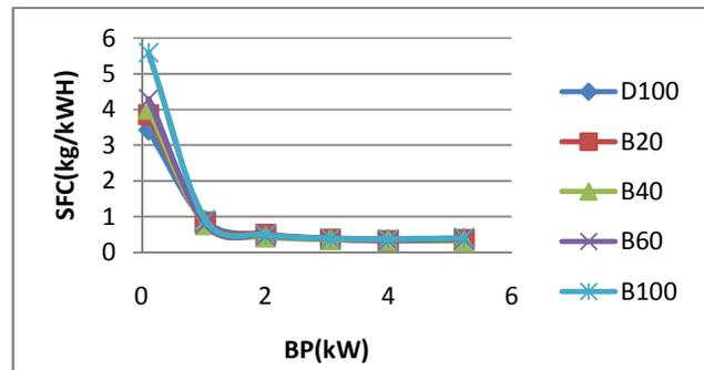
Fig 3(a): Variation of specific fuel consumption with brake power without EGR
