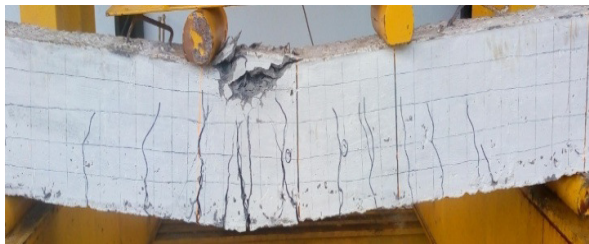
Fig. 17 Crack pattern of control beam
