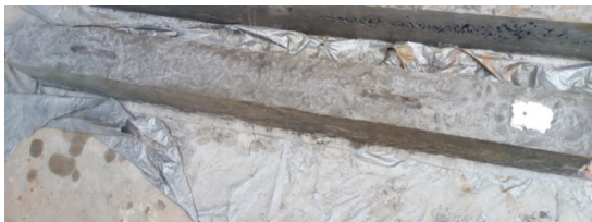
Fig. 3 Control beam casted
