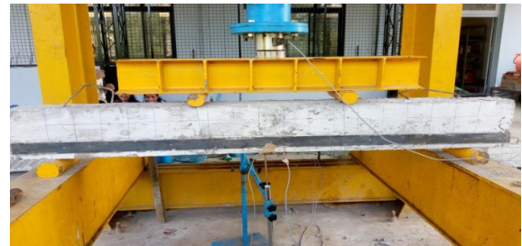
Fig. 10 Test set up for RC Beam with web bonded steel plates
