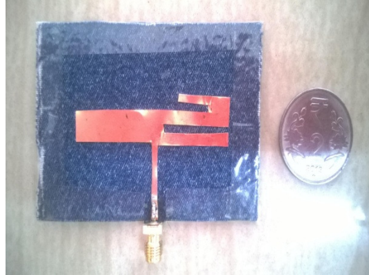
Figure 5: View of the Fabricated Wearable Antenna
