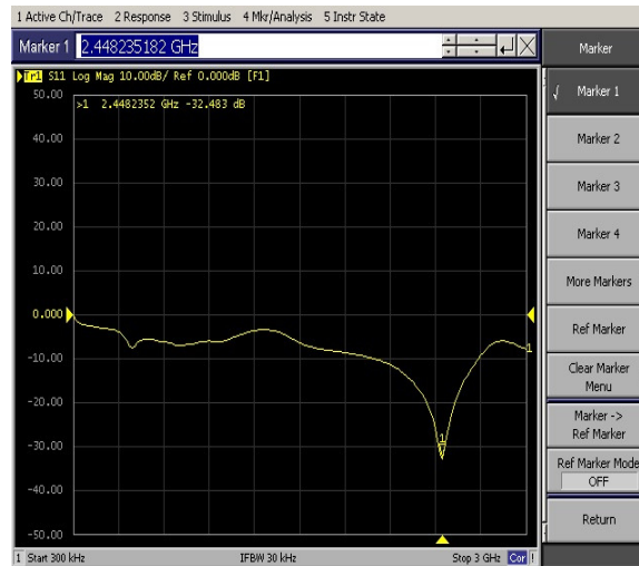
Figure 6: Network Analyzer Test Results of the Antenna
