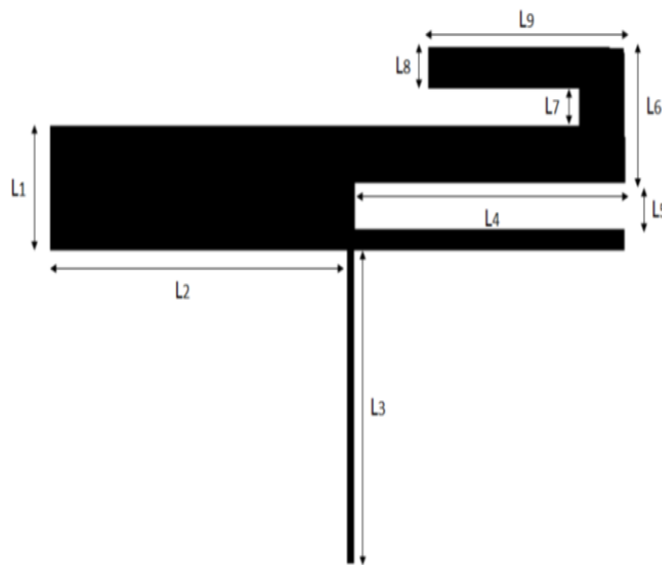
Figure 1: Proposed Wearable Antenna Design
