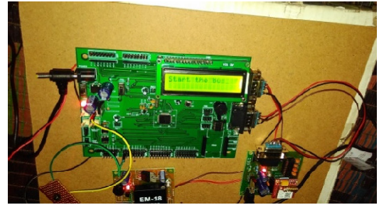
Fig 10: Bus unit with GSM and RF reader interfaces
