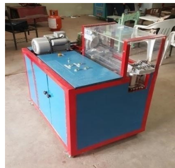
Figure 5. Completed Electrically Controlled Bearing Puller
