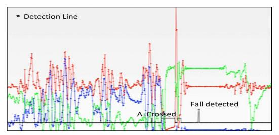
Figure 4. Pre-fall signals and fall detection confirmation
