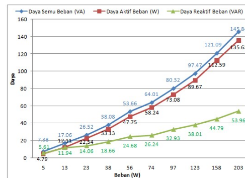
Fig. 4 Charges Against Pseudo Power, Active Power and Reactive Power Inverter Without load
