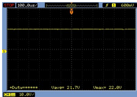
Figure 14: The output voltage of the converter
