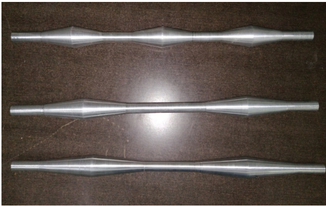
Fig.Actual V-shaped Aluminium Turbulator
