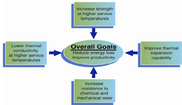
Fig. 2.1. Improving refractory materials for improved energy efficiency
