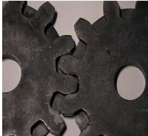
Figure 1 Gear teeth meshing.[1]
