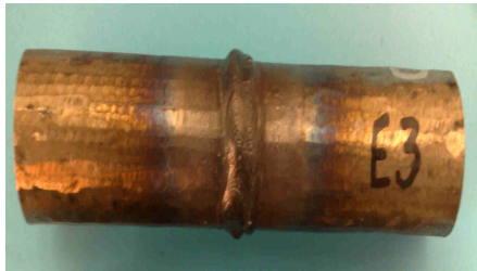
Figure 1. Point welded E3 sample, thermic untreated [1].
