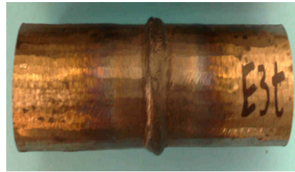
Figure 2. Point welded E3 sample, thermic treated [1].
