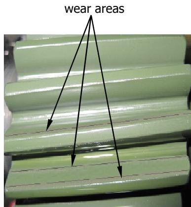
**Figure 1.** Xylan 1052 coated gear with incipient wear [15]
