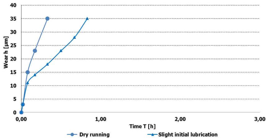
**Figure 7.** Wear evolution at a load of 120 N and a sliding speed of 2.910 mm/s
