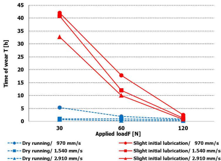
**Figure 3.** Evolution of wear time depending on applied load
