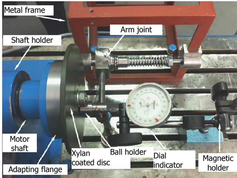
**Figure 2.** Ball-on-Disk tribometer
