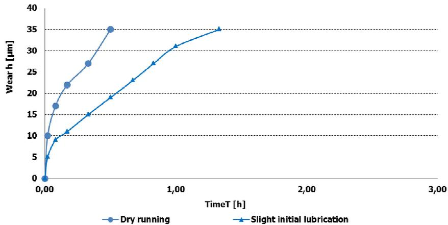
**Figure 6.** Wear evolution at a load of 120 N and a sliding speed of 1.540 mm/s
