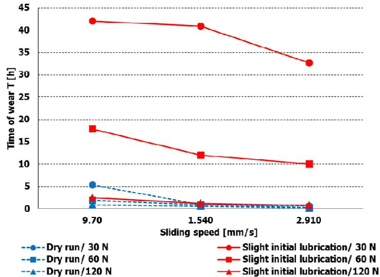
**Figure 4.** Evolution of wear time depending on sliding speed
