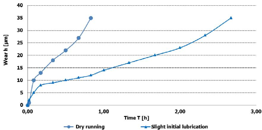
**Figure 5.** Wear evolution at a load of 120 N and a sliding speed of 970 mm/s
