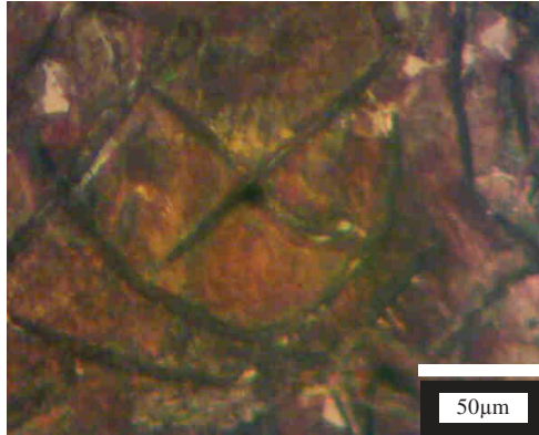
Figure 1. Photomicrograph of Specimen A, a representative of FBD etched in 2% Nital.
