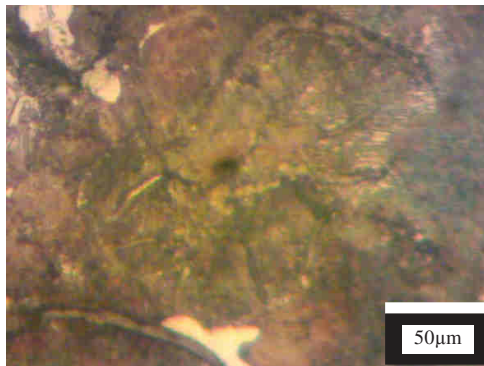
Figure 2. Photomicrograph of LFBD when polished and etched with 2% Nital
