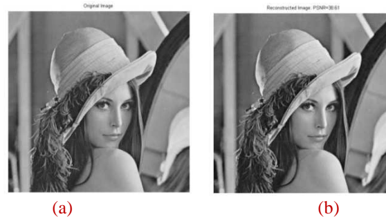
Figure 5: Compression by Dropping 28 DCT Coefficients. (a) Original Lena Image (b) Reconstructed image (PSNR=38.61)
