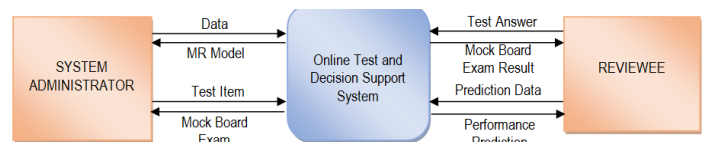
Fig. 4. Context-Level DFD of the developed OTDSS
