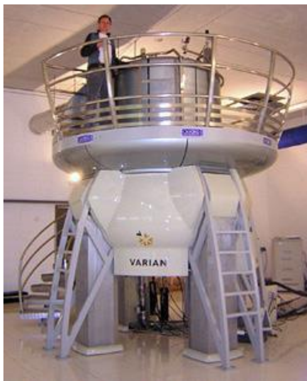
Figure 9: Nuclear magnetic resonance spectroscopy (A 900 MHz NMR instrument with a 21.1 T magnet at HWB-NMR, Birmingham, UK)
