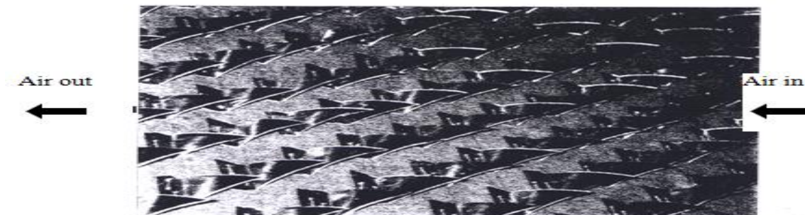
Photograph 1: Layout with DCL1 type baffles
