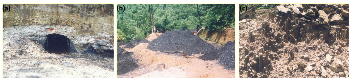
Fig. 2 | Coal mining in the study site. a: Rat-hole, b: Dumping of coal, c: Coal mine spoil.
