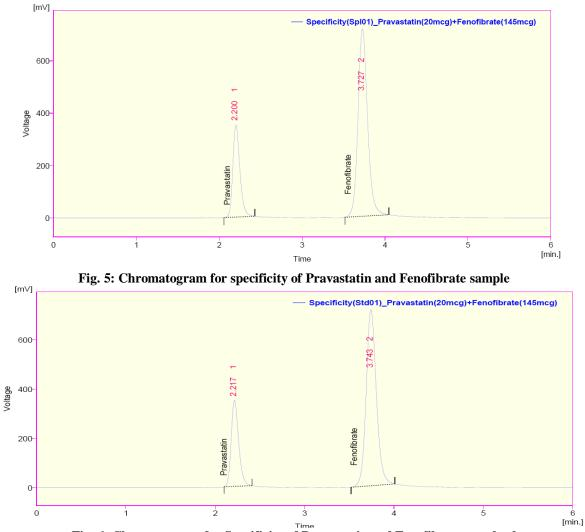
Fig. 6: Chromatogram for Specificity of Pravastatin and Fenofibrate standard
