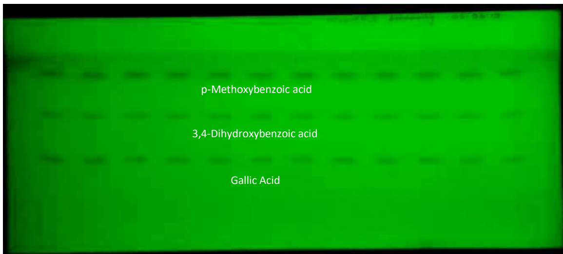
Fig. 4: HPTLC plate for Reproducibility of standards Track 1 to 12: Standard mixture of different concentrations
