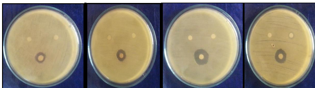
Fig.6. (A): zone of inhibition for CZO and pure ZnO against E.coli, S.aureus
