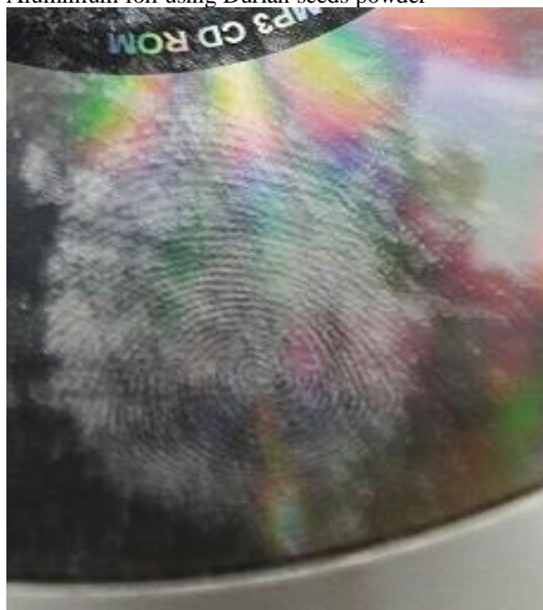
Fig 3: Visualization of latent fingerprints on written surface of CD using Durian seeds powder
