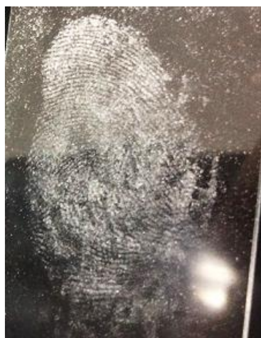
Fig 12: Visualization of latent fingerprints on microscope slide using Durian seeds powder
