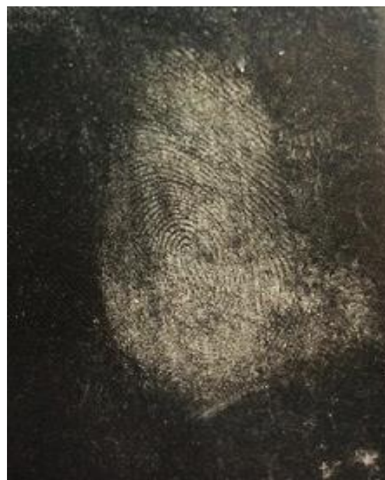
Fig 10: Visualization of latent fingerprints on translucent sheet using Durian seeds powder
