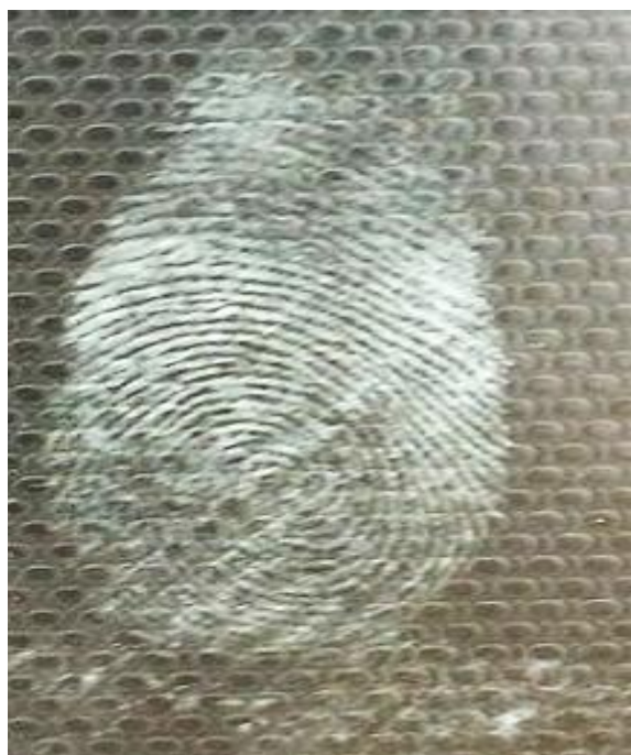
Fig 9: Visualization of latent fingerprints on steel using Durian seeds powder
