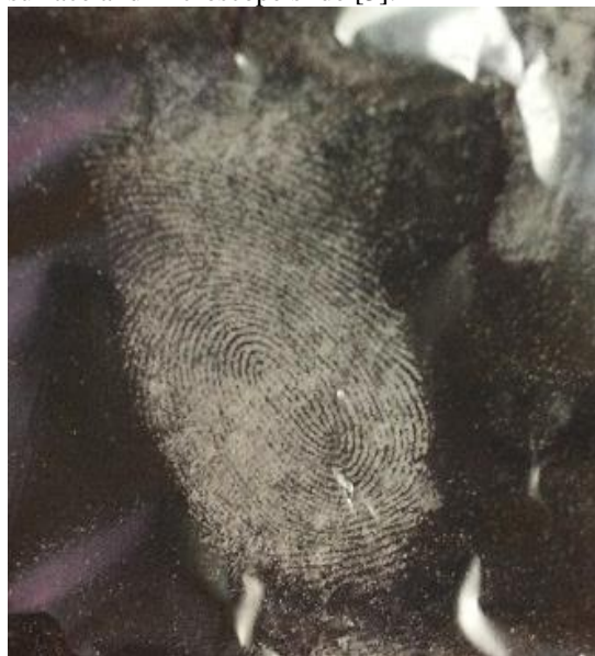
Fig 1: Visualization of latent fingerprints Aluminium foil using Durian seeds powder
