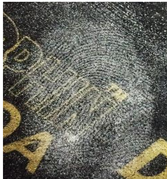
Fig 2: Visualization of latent fingerprints on Carbon paper using Durian seeds powder
