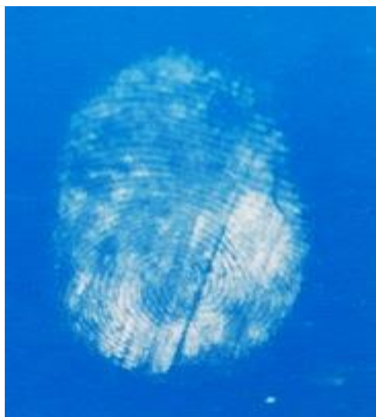
Fig 5: Visualization of latent fingerprints on painted steel using Durian seeds powder
