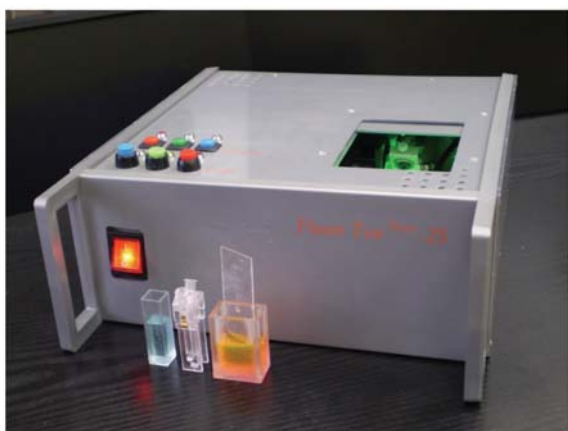
Fig. 6. Portable laser-based fluorometer FluoroTestNano-2S
