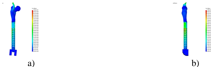
Figure 31 – Distribution of the stress-deformity state of the model with the 5° elevation angle between the upper and the middle parts of the implant, 296 mm module length, and the 30° angle between the femur axis and the knee joint load line a) front view; b) sagittal view;
