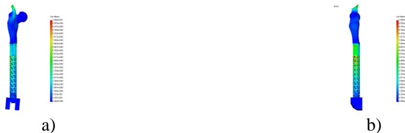
Figure 30 – Distribution of the stress-deformity state of the model with the 5° elevation angle between the upper and the middle parts of the implant, 296 mm module length, and the 0° angle between the femur axis and the knee joint load line a) front view; b) sagittal view;
