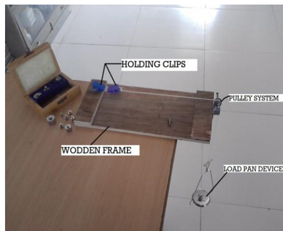
Fig 1: The tensiometer used to measure the tensile strength
