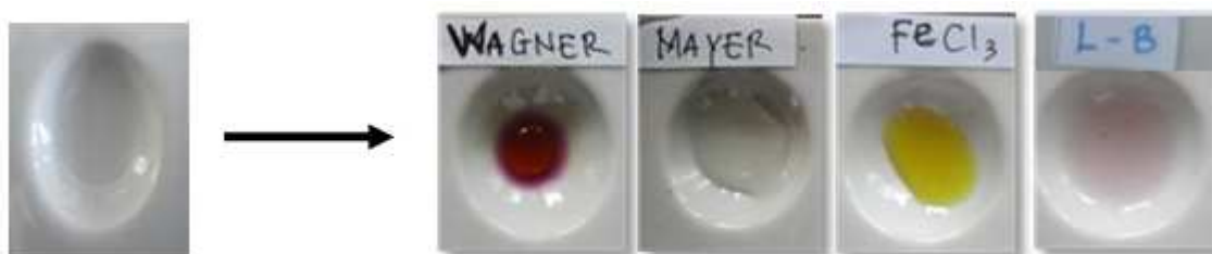
Figure 5: Color Test Results (a) Before the Addition of Reagents (b) After the Addition of Reagents
