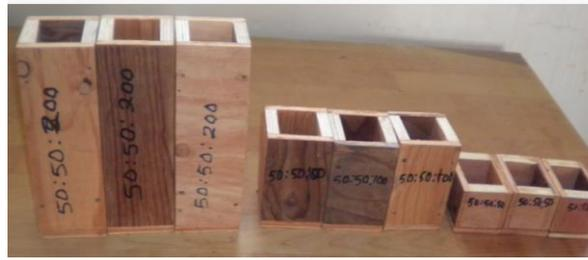
Figure 2.1: Photograph of formworks showing dimensions 50 x 50 x 200 mm and below
