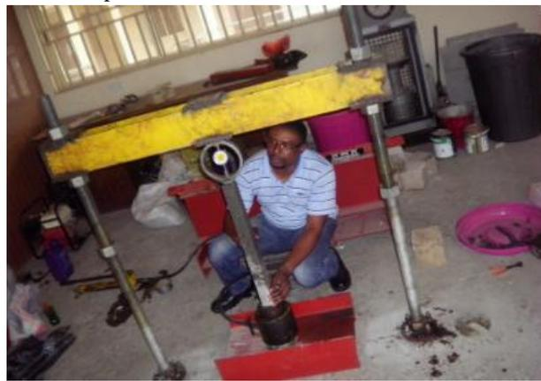
Figure 2.3: a photograph showing the crushing of one of the column samples
