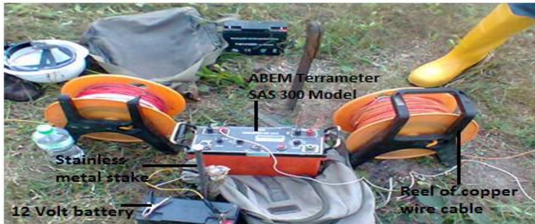
Figure 2: Showing the Field work operational instruments for VES survey
