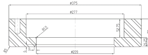
Figure 6: Geometrical dimensions of porthole flange
