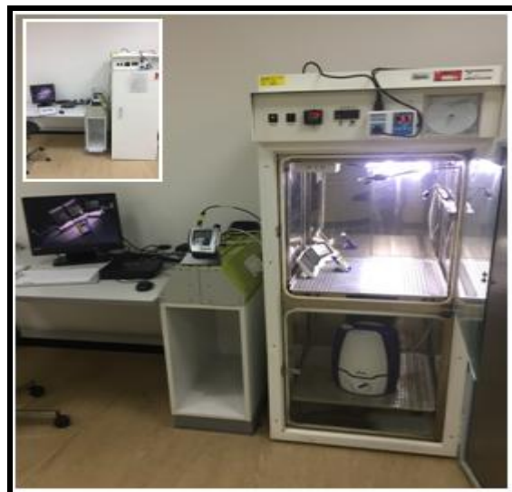
Figure 2: Actual photo for the developed humidity calibration system
