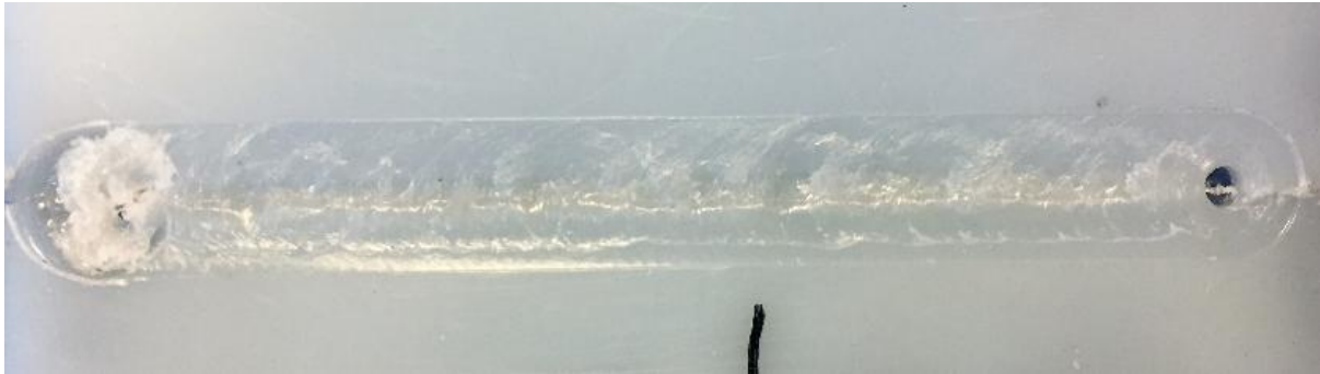
Figure 7: (Shoulder 25 mm and pin 6 mm), Surface image of welded specimens at a feed rate of 45 mm / min and 900 rpm.
