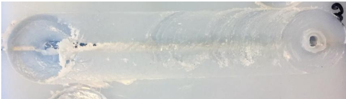
Figure 10: (Shoulder 30 mm and pin 5 mm), Surface image of welded specimens at a feed rate of 45 mm / min and 900 rpm.
