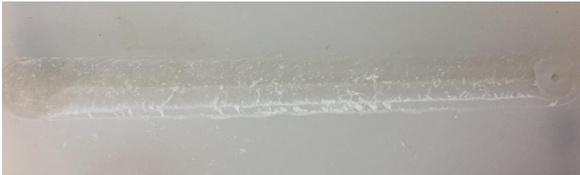
Figure 3: (Shoulder 20 mm and pin 5 mm), Surface image of welded specimens at a feed rate of 45 mm / min and 900 rpm.
