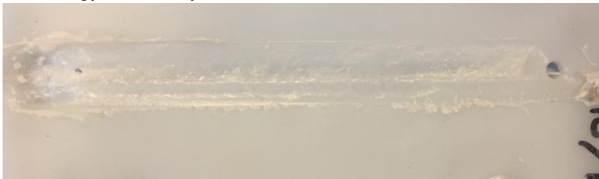
Figure 6: (Shoulder 25 mm and pin 5 mm), Surface image of welded specimens (at a feed rate of 45 mm / min and 900 rpm).
