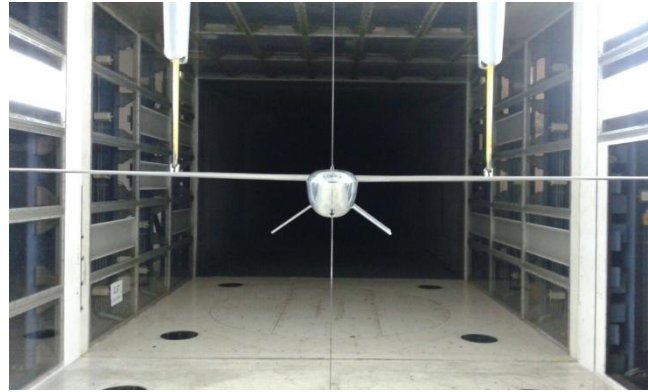
Figure 3: UAV model installed in the test section
