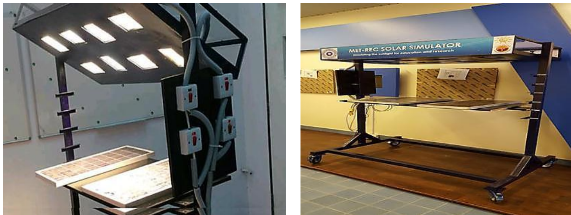
Figure 7: Experimental rig of solar simulator and lamps arrangement
