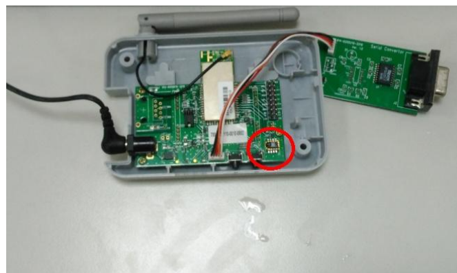
Figure 3-1: Diagram of sensor on WSN for temperature and humidity monitoring
