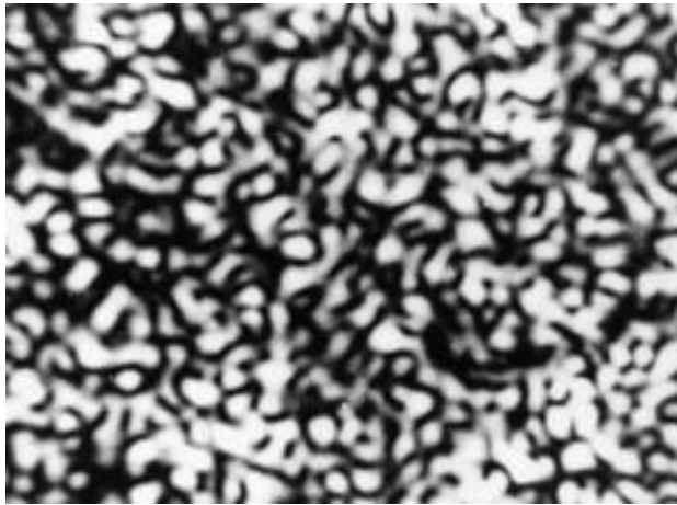
Fig. 1. Speckle pattern in the field of diffraction of a laser beam on a rough surface
