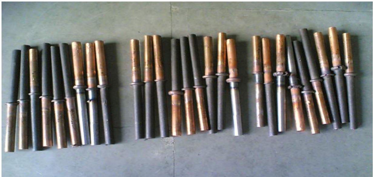
Fig. 3. Friction welded pieces at different levels of process parameters
