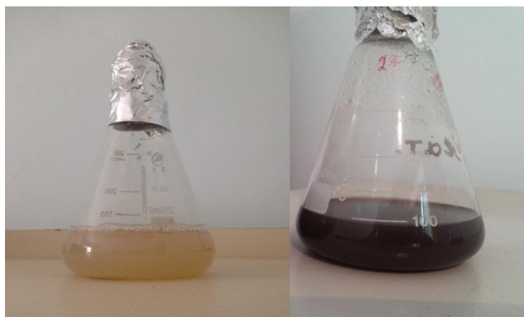
Fig.1. Change in the color of the reaction during the formation of silver nanoparticles
