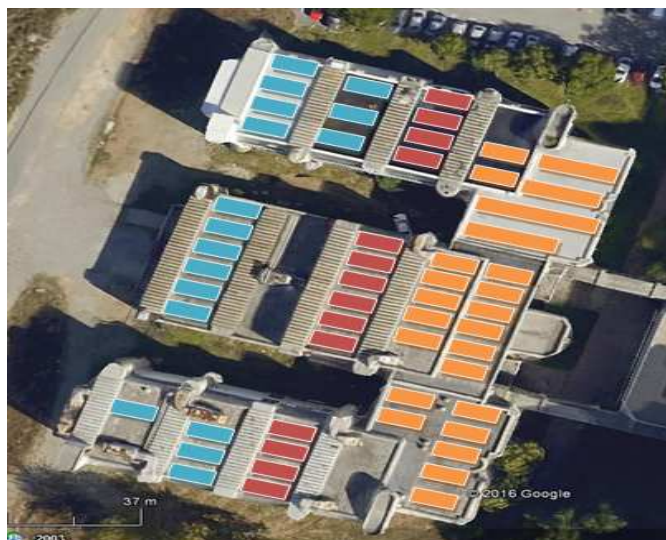
Fig. 3. Roof PV power plant (PV power plant 1- orange PV modules FN modules; PV power plant 2 – red PV modules; PV plant 3 – blue PV modules)
