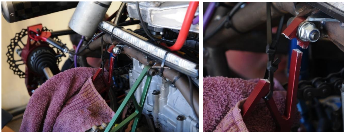
Fig. 3. Transmission support damage of the Formula Student car
