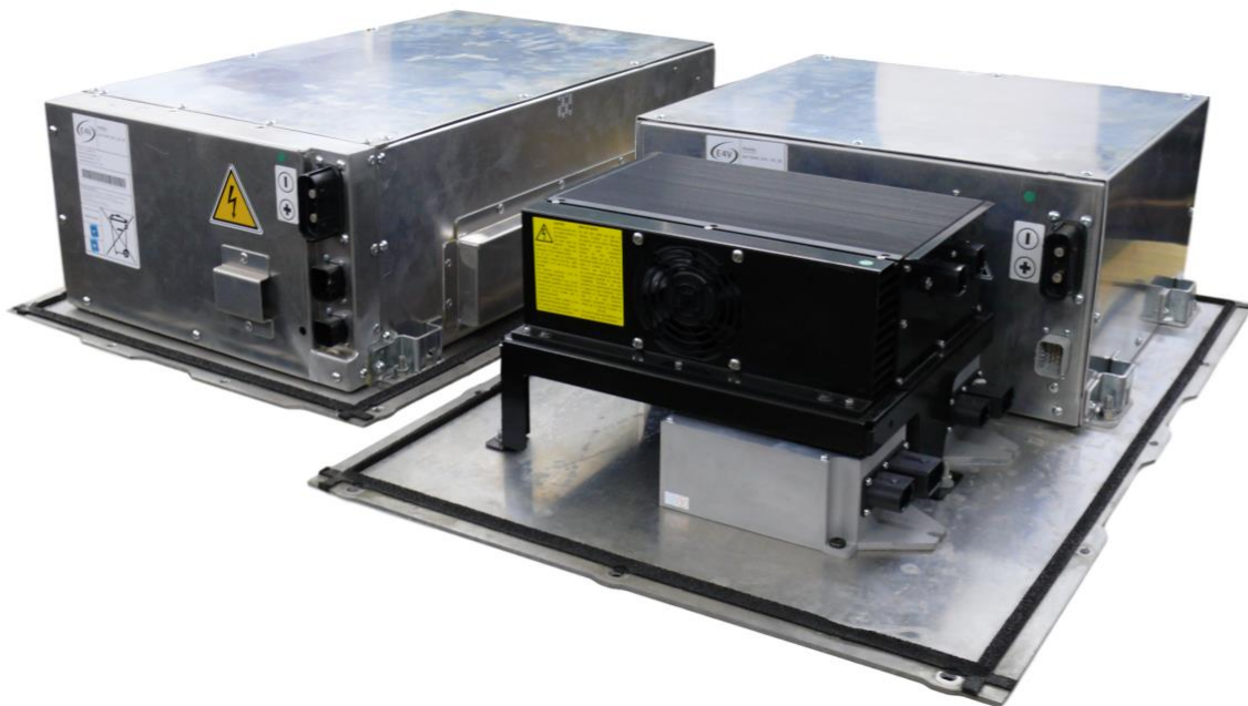
Fig. 6. View of the battery packs, the charger and the DC/DC converters
