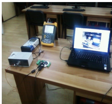
Fig. 5. Experimental setup, simulating the wind turbines vibrations monitoring.
