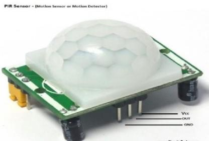
Fig.-1 shows the diagram of PIR Sensor
