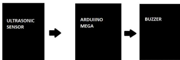
Fig.4: Door Alarm using Arduino and Ultrasonic Sensor
