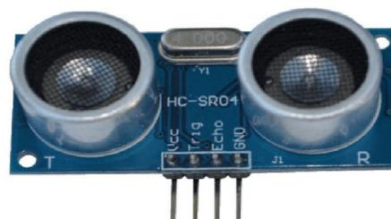
Fig.3: Ultrasonic Sensor
