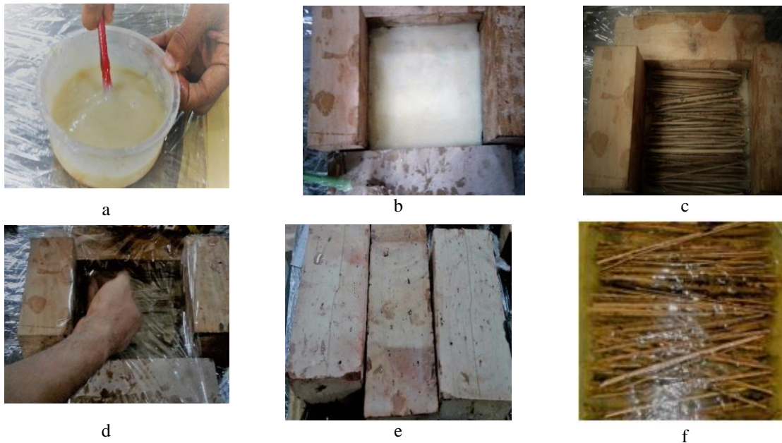
Fig. 3 Complete sequential process for fabrication (a) Mixing resin and fiber in appropriate proportion (b) Pouring of mixer in to the mold (c) Placing fiber on the mixture (d) Wrapping with masking tape (e) Force applying manually (f) 72 hours later
