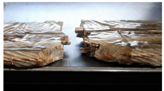
Fig. 9 The edges after impact test
