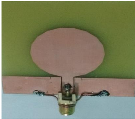
Fig. 8 Fabricated reference antenna structure
