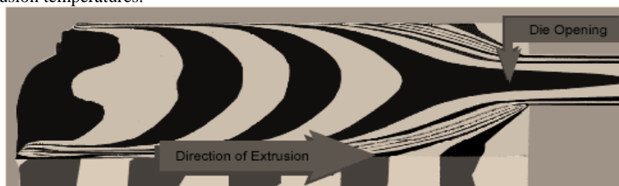
Fig. 3 View of Extrudate Passing through the Die Opening
