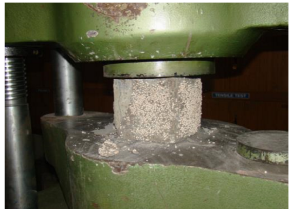
Fig.10 Cube tested for its compressive strength in UTM
