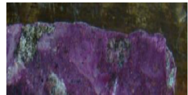
Fig.12 Carbonation depth of ZPC at 28 days CO 2 exposure – 0mm
