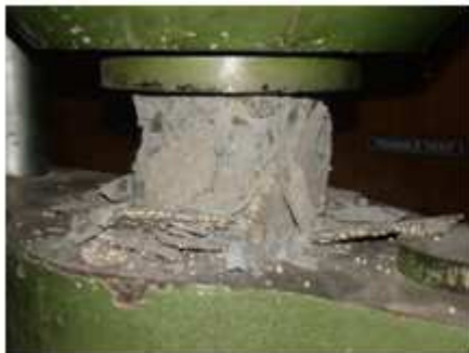
Fig.16 Cube tested for its Compressive Strength after Fire exposure
