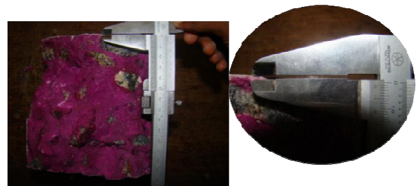
Fig.14 Carbonation depth of ZPC at 56 days CO 2 exposure – 1mm
